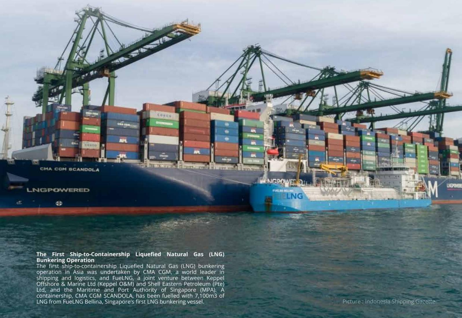
**The First Ship-to-Containership Liquefied Natural Gas (LNG) Bunkering Operation**
